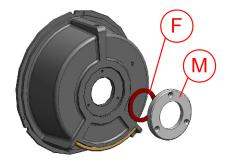
If the felt ring is worn, remove the grinding set. Remove the metal ring (M) on the rear of the grinding chamber cartridge by loosening the 3 screws and replacing the felt ring (F). Put everything back together in the reverse order. (see Chapter & Chapter 6.3 'Installing the grinding elements' on page 24)
