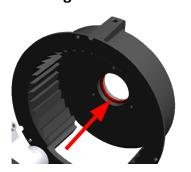
Grease the felt ring (F) in the grinding chamber cartridge every week with a few drops of machine oil.
