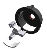
To facilitate cleaning, the grinding chamber, bottom sieve and cross beater can all be removed. For this, see Chapter & Chapter 6.3 'Installing the grinding elements' on page 24.
